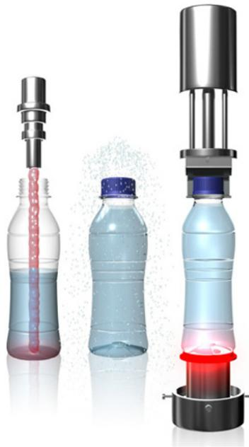
**Figure 9.4** Base re-heat diagram (courtesy of Plastipak).
